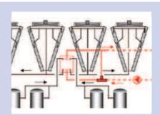
An optional heat recovery feature can be added to provide hot water to  $50^{\circ}$ C; which is useful for facility heating or hot water preheating.
