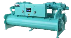
YVWH High Head HP Water to water HP VSD Screw / R1234ze Hot water up to 80°C Heating capacity: 800 to 1600 kW
