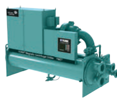
YMC² Water to water HP VSD Centrifugal Magnetic bearings R513A Hot water up to 65°C Heating capacity: 1600 to 3000 kW
