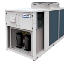
YLZ Air to water HP E.V.I 4 pipe system Scroll E.V.I / R410A Hot water up to 65°C Heating capacity: 42 to 210 kW
