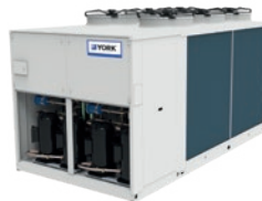
YHA Air to water HP 4 pipe system Scroll / R410A Hot water up to 60°C Heating capacity: 41 to 464 kW
