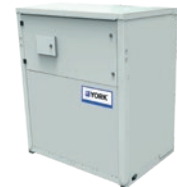
YWH Water to water HP Scroll / R134a Hot water up to 78°C Heating capacity: 44 to 301 kW
