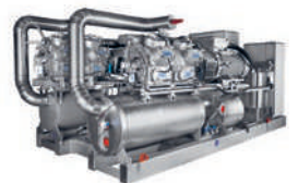
DualPAC recip 2-stages Variable-Speed Drive Reciprocating / R717 Hot water up to 90°C Heating capacity: 400 to 2900 kW
