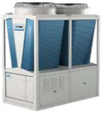
YMAE Air to water HP Scroll / R454B Hot water up to 60°C Heating capacity: 42 to 330 kW
