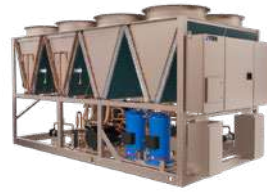
YCPB Air to water HP Scroll / R454B Hot water up to 60°C Heating capacity: 300 to 745 kW
